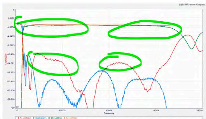
Orange and Blue - XG3 Eulex Gap Capacitor Green and Red - Single Layer Capacitor
