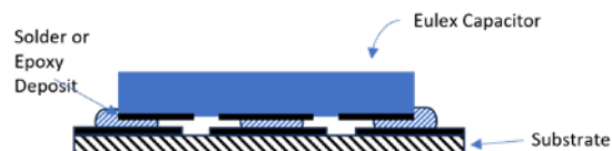
3-pad terminal Gap capacitor mounted face-down on GCPW (coplanar waveguide w/GND)
