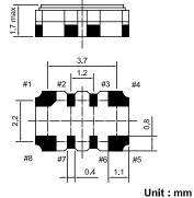
Pin Function #1 GND or N.C. #2 N.C. #3 N.C. #4 GND #5 Output
