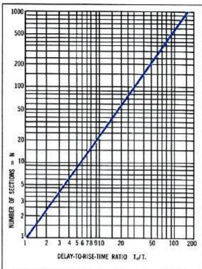
Fig. 4. The relationship between figure of merit,  $T_a/T_c = R$ , and the number of sections of a lumped constant delay line needed to achieve it,  $N = R^{1.24}$ , as plotted on log paper.
