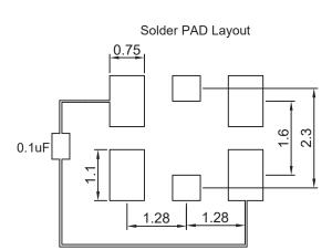
To ensure optimal oscillator performance, place a by-pass capacitor of  $0.1 \mu F$  as close to the part as possible between VCC and GND pads.
