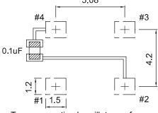
To ensure optimal oscillator performance, place a by-pass capacitor of 0.1uF as close to the part as possible between Vcc and GND PAD
