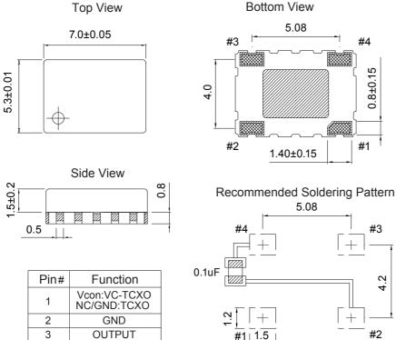
To ensure optimal oscillator performance, place a by-pass capacitor of 0.1uF as close to the part as possible between Vcc and GND PAD
