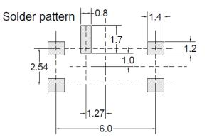
Pin function #1 Vc (EFC) #5 GND #6 Output #9 E/D or NC
