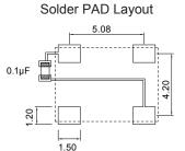
To ensure optimal oscillator performance, place a by-pass capacitor of  $0.1\mu F$  as close to the part as possible between Vdd and GND pads.
