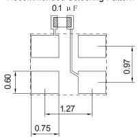
To ensure optimal oscillator performance, place a by-pass capacitor of 0.1uF as close to the part as possible between Vcc and GND PAD
