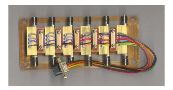
Planar Monolithics Industries Model No: SAA-218-6-093-013542 is an Array of Six Switched Bit Attenuators (AMC Model No: SBA-218-6) operating from 2 to 18 GHz. This Assembly provides Switchable RF Attenuation for Six Signal Paths. The settings will be selected by Six Digital Control Bits. The standard version of this product is Epoxy Sealed, but the Hermetically Sealed version is available for more extreme environmental requirements.
