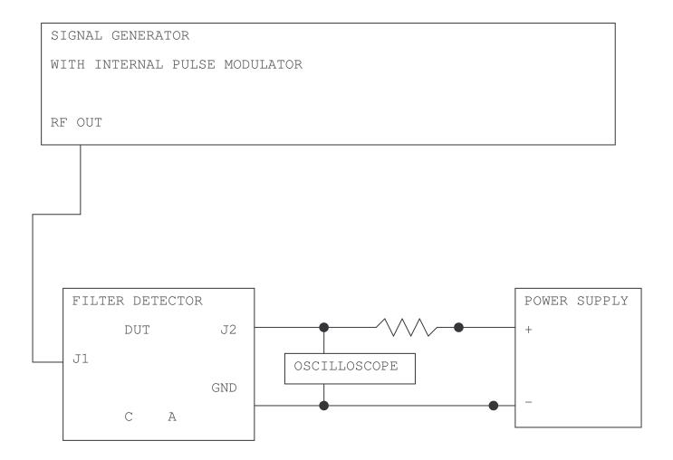
Series Resistors of 10 kohm will give 100 microamp when power supply is 1 volt above the diode voltage.
