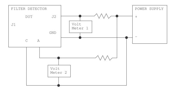
Series Resistors of 10 kohm will give 100 microamp when power supply is 1 volt above the diode voltage. Typically 1.3Volts
