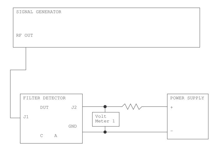
Series Resistors of 10 kohm will give 100 microamp when power supply is 1 volt above the diode voltage.
