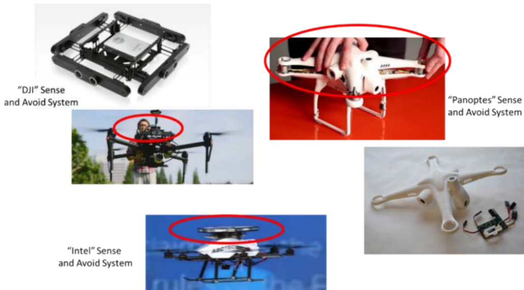
Figure 1. Sense and avoid systems presented on the market today are large compared to drone size, and expensive.
