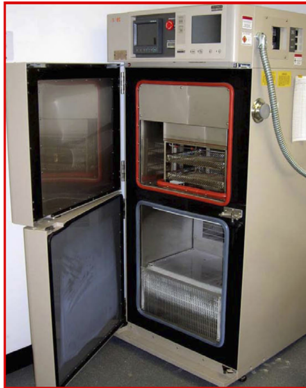
Temperature cycling MIL-STD-883G, Method 1010, Condition B
