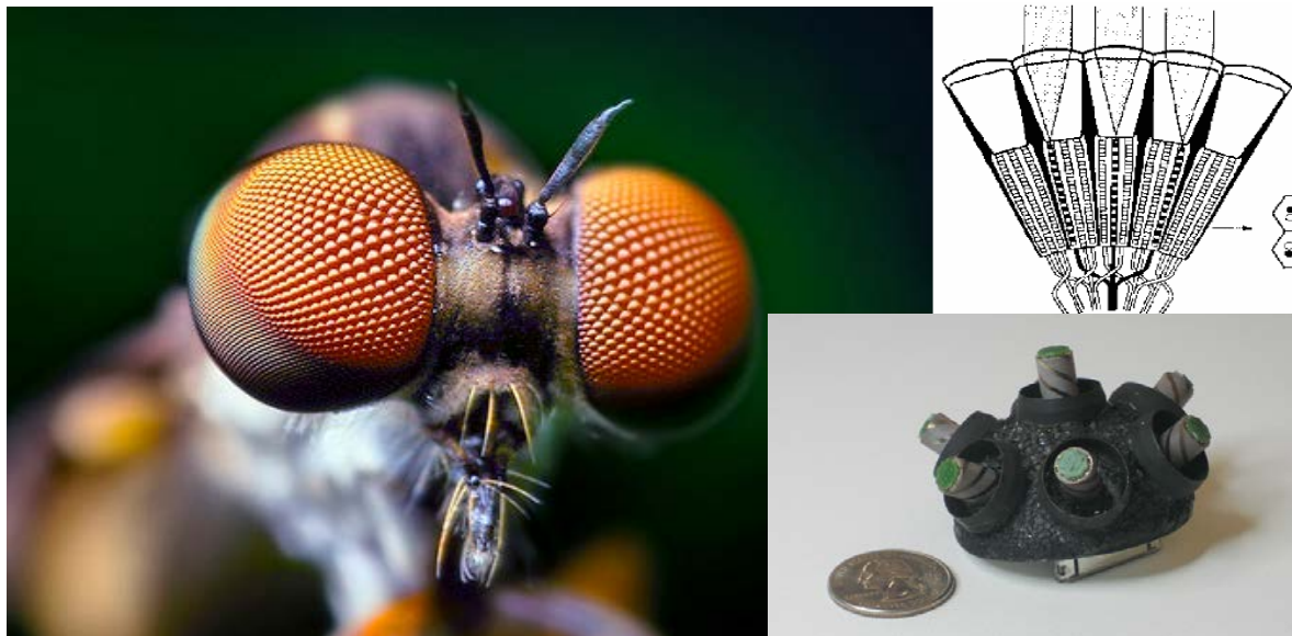
Figure 1. The fly's eye consists multiple directional optical sensors coupled with detectors. Each sensor connected to memory by separate nerve. Fly Eye antenna array concept: multiple directional antennas coupled with front end circuits and analog-digital converters in each antenna modules. Digital interface connecting all antenna modules to processor.
