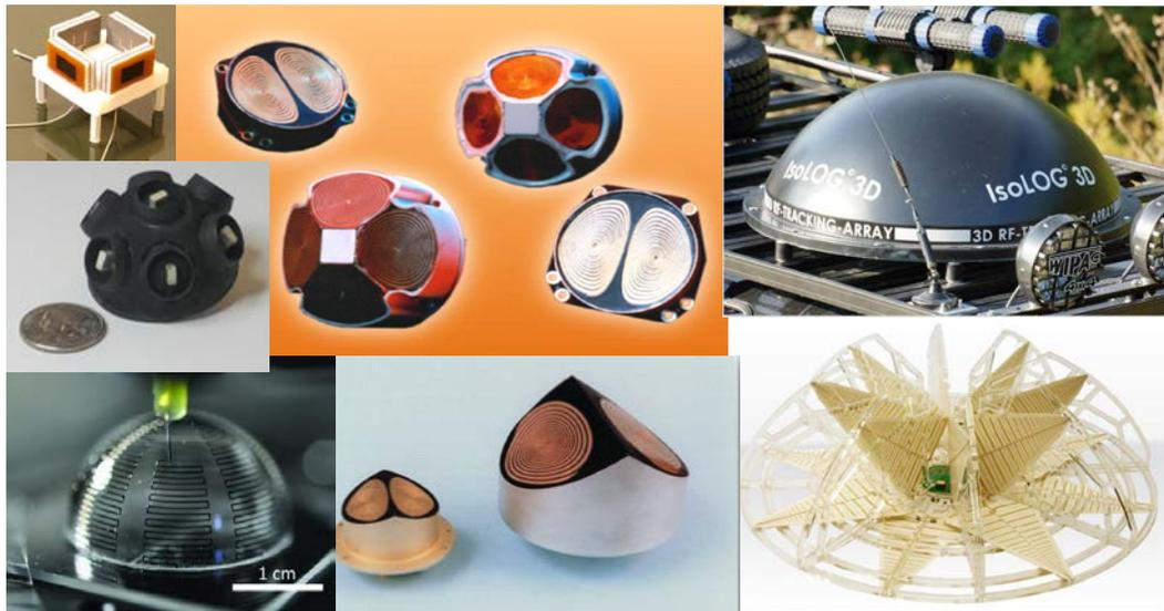
Figure 17. Ultra-wide band monopulse antenna arrays can have different size. Smallest antenna arrays can be applied for handheld bomb detection.
