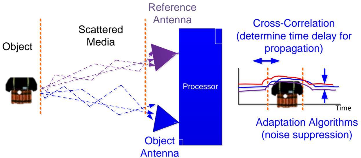
Figure 12. Additional (reference) antenna allows to separate object and scattered media signals in radar receiver. Cross-correlation and adaptation algorithms provides dramatically enhancing of image resolution.
