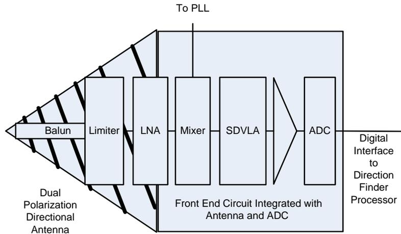
Figure 16. Wideband dual polarization directional antenna integrated with front end circuit and analog to digital converter.
