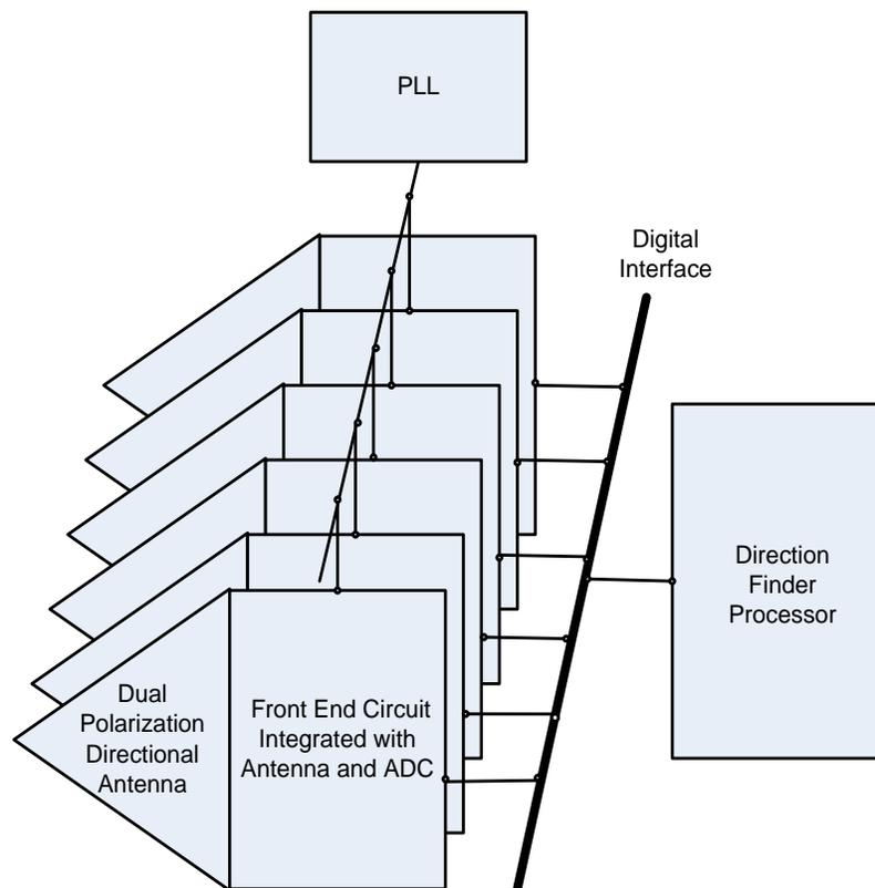
Figure 15. Block diagram of proposed IDF.
