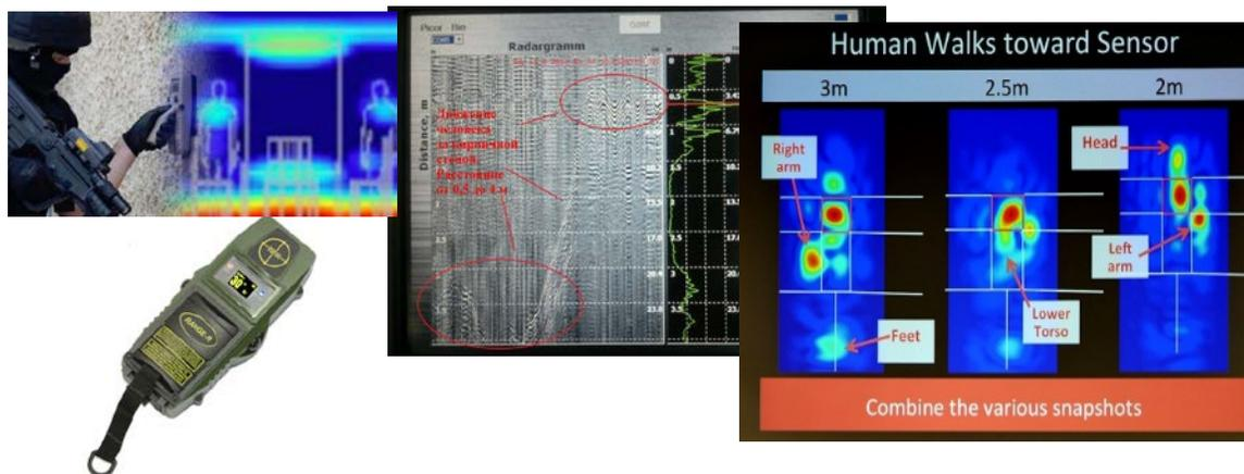
Figure 1. Existing radar imaging technologies provide only direction and range to target, or low (approx. on foot size) resolution image, where object cannot be identified with good enough probability.
