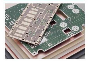
RT/duroid® 5870 and 5880 glass microfiber reinforced PTFE composites are designed for exacting stripline and microstrip circuit applications.
