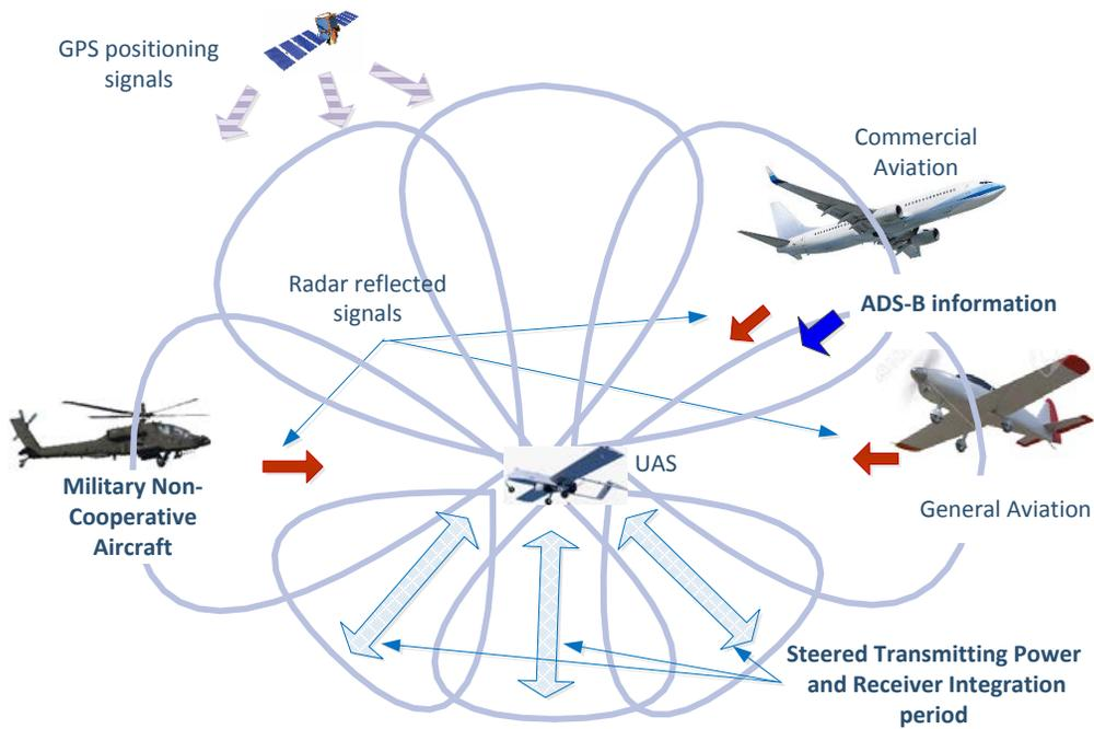
Figure 1. Concept of multibeam monopulse radar for airborne based sense and avoid system.
