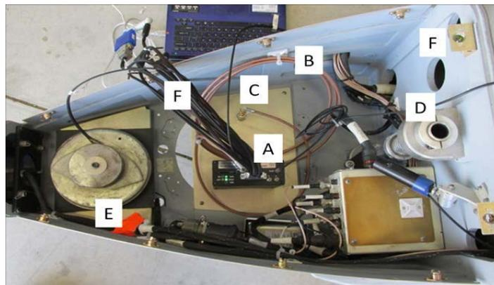
Figure 16. Installation of the AWSAS (A) in the TS-60 UAS.
