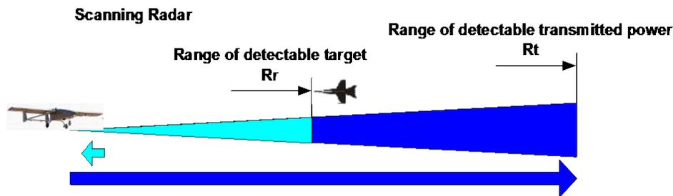
Figure 8. In regular scanning radar the range of detectable transmitted power  $R_t$  is larger for larger transmitting power and smaller beamwidth.
