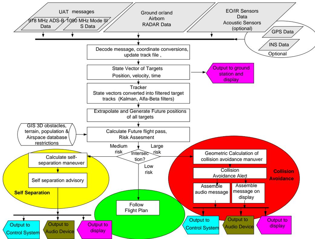
Figure 11. Open architecture ABSAA algorithm consists of three main parts including self-separation and collision avoidance.
