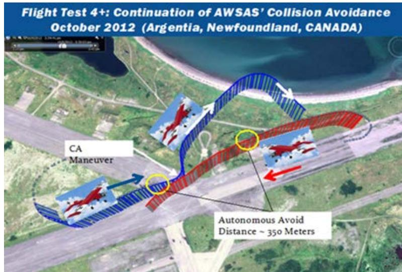
Figure 17. Collision avoidance test results with group 2 UAS. Newfoundland, Canada.
