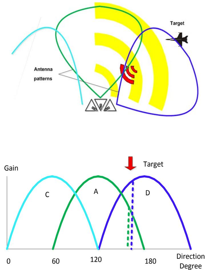
Figure 10. If the lobes of two antennas are overlapped, this signal can produce a high degree of pointing accuracy within the beam, adding to the natural accuracy of the conical scanning system.
