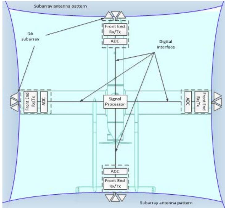
Figure 15. Sub-arrays of directional antennas coupled with Tx/Rx modules can be loosely distributed over UAS perimeter and connected with radar signal processor by digital interface.
