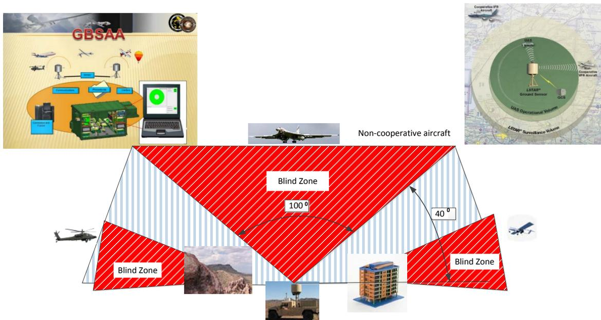
Figure 2. Ground based sense and avoid system with LSTAR (V)3 radar by SRC Inc. providing limited area of observation with large blind zones, where non-cooperative aircraft invisible.
