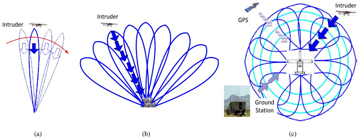
Figure 7. Scanning radar (a), monopulse radar (b) and Fly Eye radar (c).
