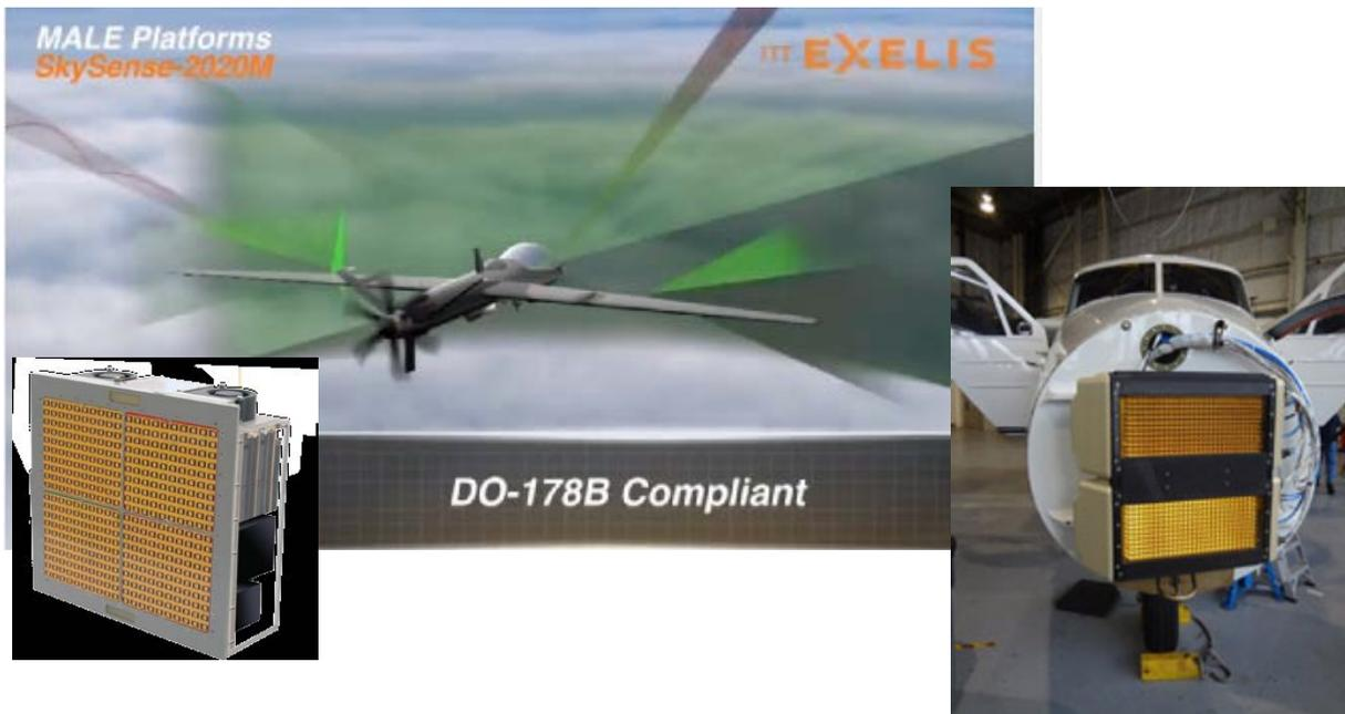
Figure 3. ABSAA systems with phased antenna array designed by Excelis Inc. (on left) and MIT LL (on right).
