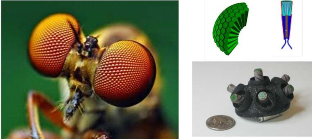
Figure 6. Fly Eye antenna array with angular shifted array of directional antennas.
