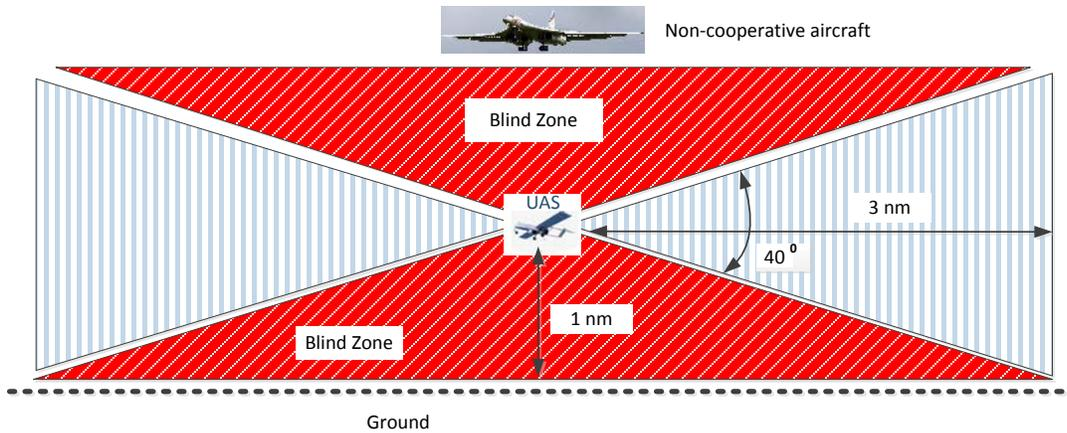
Figure 4. Airborne Based Sense and Avoid System (ABSAA) with **scanning** radar can provide limited area of observation.
