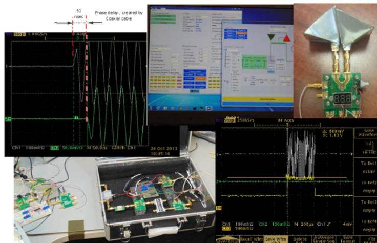
Figure 14. Test of radar receiver designed by Dr. Pavlo Molchanov as PI in Air force FA8650-13-M-2373 project. Measurement of time delay between ADS-B messages. The frequency of radar signals (multi-frequency or special shape signals optional) can be synthesized with a Phase Locked Loop (PLL) or optionally ADS-B messages can be used as radar signals.
