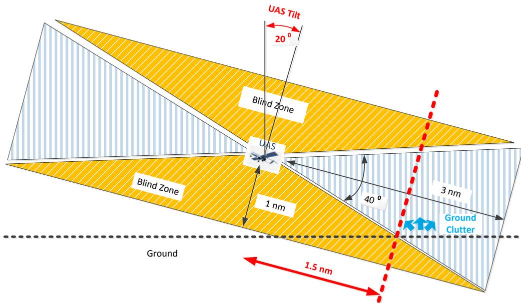
Figure 5. Small (20 degree) tilt of UAS with ABSAA scanning radar will decrease radar range approximately to 50%.
