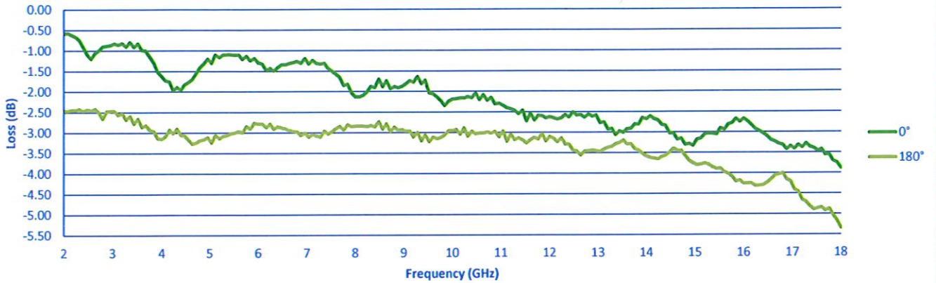
Insertion Loss at Phase Settings
