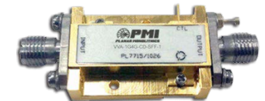
1 to 4 GHz, Voltage Variable Attenuator
