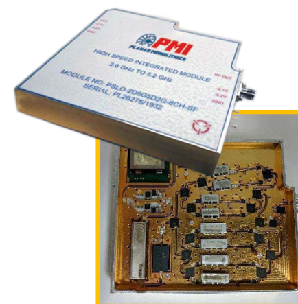
2.6 to 5.2 GHz 8 Channel Selectable LO Frequency Source
