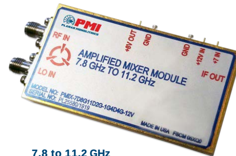
7.8 to 11.2 GHz Down Converter Module
