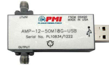
0.05 to 18 GHz, 12 dB Gain USB Powered LNA
