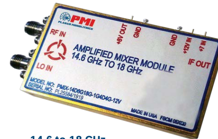
14.6 to 18 GHz Down Converter Module
