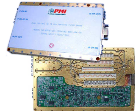
Double Sided, 0.01 to 18 GHz 6 Channel Switch Filter Bank
