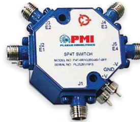
0.1 to 20 GHz SP4T Absorptive Switch
