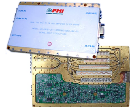
Double Sided, 100 MHz to 18.0 GHz 6 Channel Switch Filter Bank
