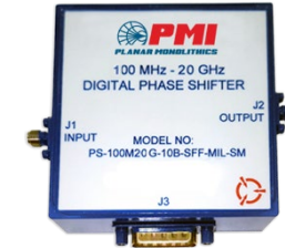
0.1 to 20 GHz, 360° 8-Bit Digital Phase Shifter
