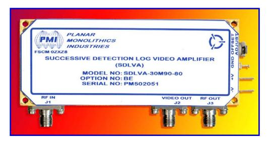
PMI Model SDLVA-30M90-80 is a Successive Detection Log Video Amplifier (SDLVA) that is designed to operate over the Frequency Range of 52 MHz to 68 MHz. The Input Dynamic Range is from -14dBm to -84dBm while the Limited IF output is 0dBm and the Maximum RF Input power is 0dBm. The Log Video Rise and Settling Times are 500nS Maximum and the Slope is at 55mV/dB with a Propagation Delay of 10nS Typical. The Size is: 3.75" X 1.50" X 0.50".
