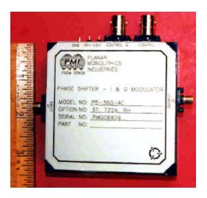
**PLANAR MONOLITHICS** INDUSTRIES, INC. Produces the PMI Model No: PS-360-AC which is an Analog Controlled Phase Shifter / High Speed I & Q Modulator which has been optimized for 3.5 to 6.5 GHz Frequency Range (other Frequency **Ranges** are available). It is designed to have low spurious harmonics, insertion loss and a VSWR of only 2.0:1. It operates with  $\pm 15$ VDC and it's size is 3.25" x 3.25" x 0.85".
