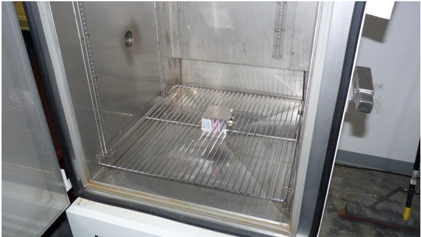
Photograph 1: MIL-F-18770E Humidity Test Configuration
