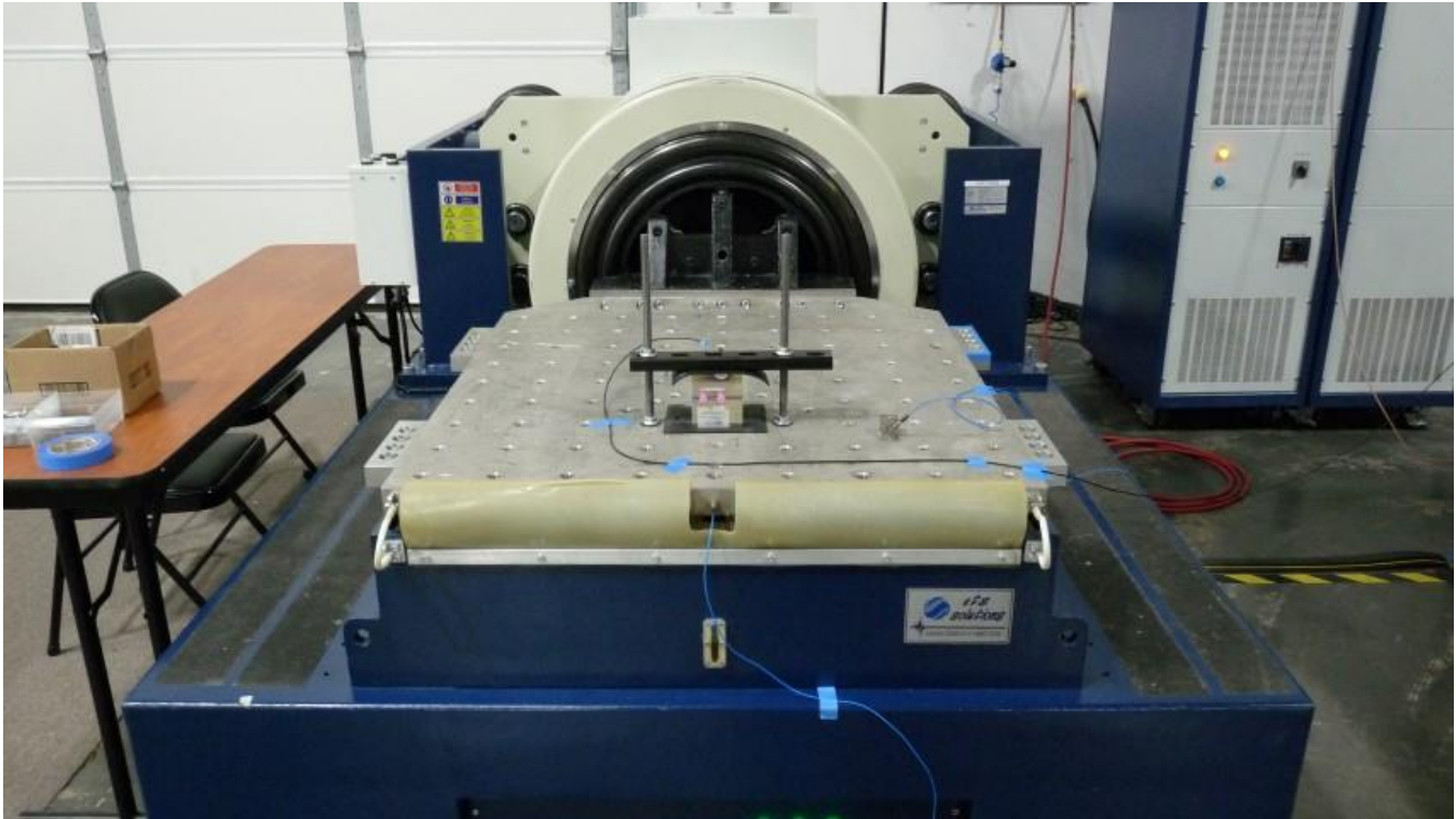
Photograph 2: MIL-STD-167A Vibration & Shock Test, X-Axis Configuration
