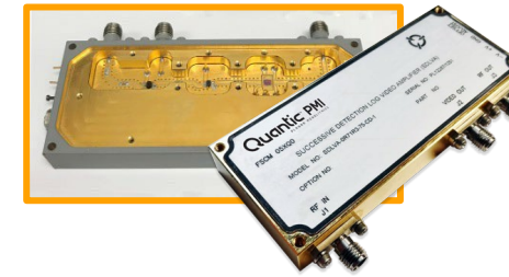
0.7 to 1.3 GHz IF Logarithmic Amplifier (SDLVA)
