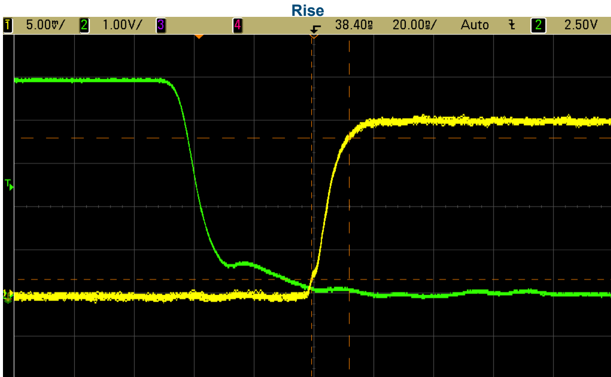
RF Signal = Yellow Trace, TTL Signal = Green Trace Switching Speed On = 50 ns
