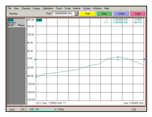
\*The phase setting on the VNA increases from  $0^{\circ}$  to  $180^{\circ}$ . Once the phase is past  $180^{\circ}$  it is plotted as -180° and then becomes less negative until it reaches  $0^{\circ}$  again (360° shift). For example  $90^{\circ}$  is  $90^{\circ}$ ,  $180^{\circ}$  and  $-180^{\circ}$  are  $180^{\circ}$ ,  $-90^{\circ}$  is  $270^{\circ}$ , and  $-1^{\circ}$  is a  $359^{\circ}$  shift.
