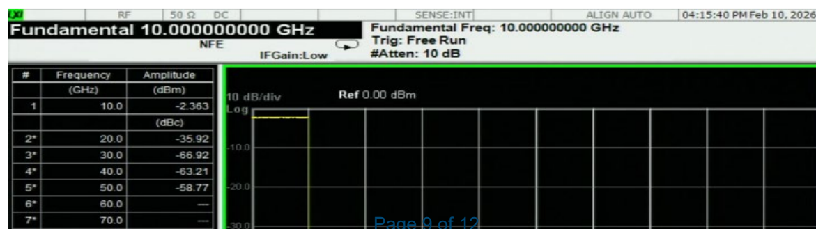
Second Harmonics Vs Frequency @ -30 dBm Input Power Fundamental 10 GHz
