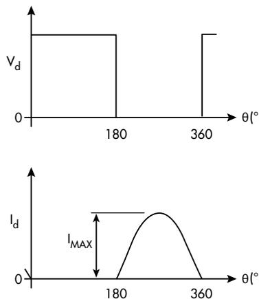
1. The plot shows a Class F drain-voltage and drain-current waveform.
