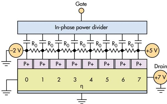
5. This diagram of a Grayzel JFET model shows each p-n junction biased at  $-2$  V dc and with in-phase RF voltage provided by means of an in-phase power divider.
