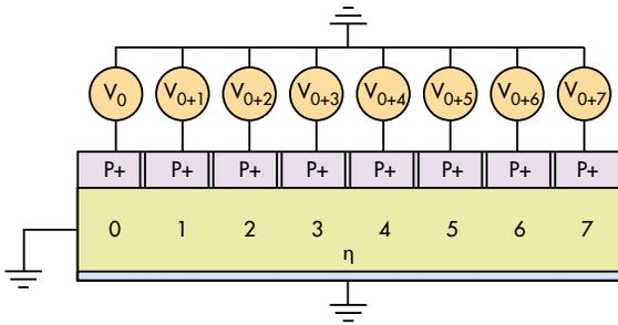
4. Each p-n junction in this Grayzel JFET model is reverse-biased at voltage  $V_0$ .
