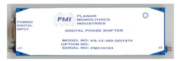
PMI MODEL PS-12-360-QQ1470 IS AN ANALOG PHASE SHIFTER WITH A MINIMUM PHASE SHIFT OF 360° AND A FREQUENCY OF OPERATION OF 1.0 to 2.0 GHz, OTHER FREQUENCY BANDS AVAILABLE UP TO 18 GHz. THE INSERTION LOSS IS 5.5 dB TYPICAL AND SWITCHING SPEED IS 200nS TYPICAL. THE PHASE SHIFTER USES TTL BINARY CONTROL WITH AN LSB OF 1.41°. THE POWER SUPPLY IS  $\pm 15$  VDC AND THE SIZE IS 7.75" X 2.5" X 1.00".
