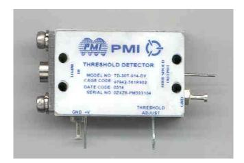
Planar Monolithics Industries Model No: TD-30T-914-DX is a High Speed Threshold Detector Designed to Operate over the 9 to 14 GHz Frequency Range, with an Adjustable Threshold Level of -18 dBm to +5 dBm, and a Typical VSWR of 2.0:1 (2.5:1 Maximum). This unit comes in a very small size with a Field Removable GPO Connector on the Input and a Solder Pin on the Output.
