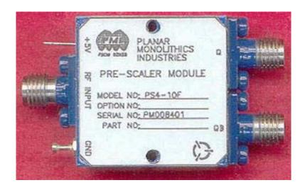
THE PMI MODEL PS4-10F IS A HIGH SPEED, PRE-SCALER FREQUENCY DIVIDER. THE MODEL ILLUSTRATED IS OPTIMISED FOR 4.0 TO 10.0 GHz AND FEATURES A HIGH INPUT SENSITIVITY OF -10dBm @10 GHz @ 25°C. MAXIMUM RF INPUT POWER IS +15 dBm AND THE SIZE IS 1.00" X 1.00" X 0.50".
