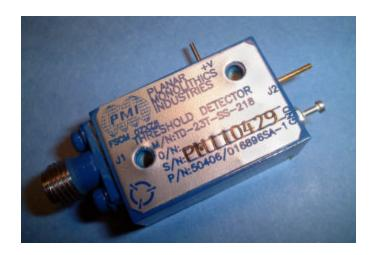
PLANAR MONOLITHIC INDUSTRIES, INC. MINIATURE 2 TO 18 GHz THRESHOLD DETECTORS, PMI MODEL No: TD-23T-SS-218 HAS AN INPUT OPERATING RANGE OF -18dBm TO -23dBm OVER THE FULL FREQENCY RANGE. THE THRESHOLD LEVEL IS INTERNALLY FIXED TO PROVIDE A MINIMUM SIGNAL LEVEL OF -23dBm. THE INPUT VSWR IS <2.5:1 AND THE RESPONSE TIME IS <100μS. THE DEVICE USES A SINGLE +12vdc DC SUPPLY AND THE SIZE IS 1.00" X 0.65" X 0.40".
