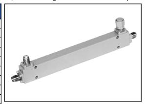
The Model C1-A85 Series is one of RD Microwaves new Taperline products for broadband flat coupling values over the full range of 0.5-12.4 GHz. The frequency sensitivity is included in the coupling accuracy specification over the full frequency range. The unit uses a stripline continous taper construction with an RFI compression sealing system for temperature insensitive performance and RF leakage control.
