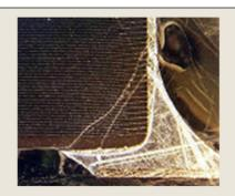
Fig. 2 Ceramic Capacitor "Cracking"
