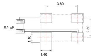
To ensure optimal oscillator performance, place a by-pass capacitor of 0.1uF as close to the part as possible between Vcc and GND PAD
