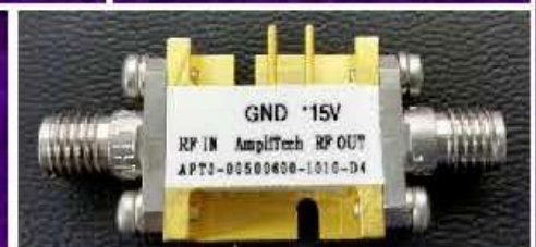
APT3-00500600-1010-D4 Wideband Amplifier (NF<1.0dB) for PCS, GPS, WiFi & 4G/5G
