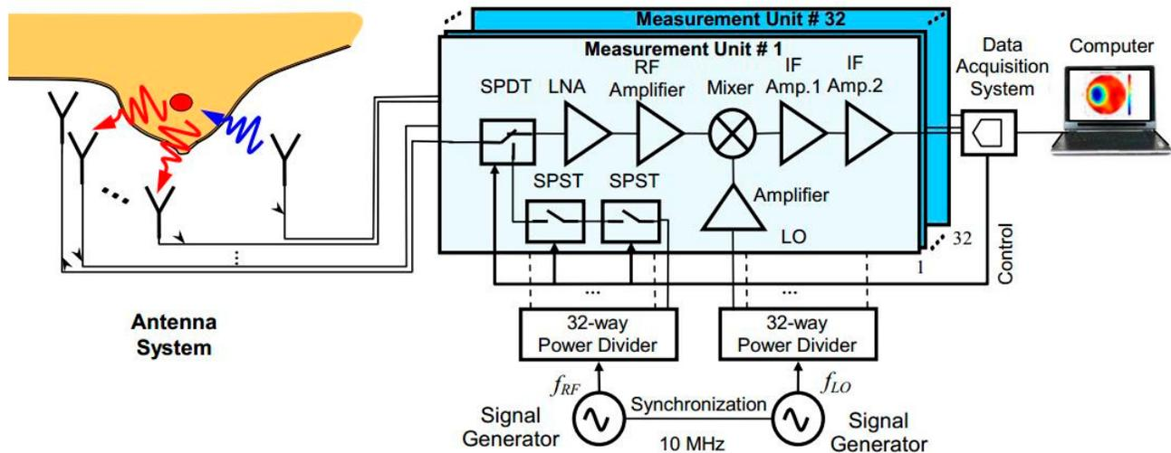
**Figure 1:** Schematic block diagram of MW imaging using UWB antenna sensor (13).
