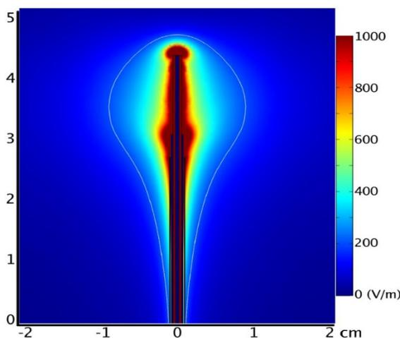
**Figure 2:** Heating pattern around a triaxial MW ablation antenna. Note that the zone of active heating is nearly 2 cm in diameter and no ground pads are needed. This larger zone of heating results in better performance near blood vessels and improved multiple-antenna capabilities (16).
